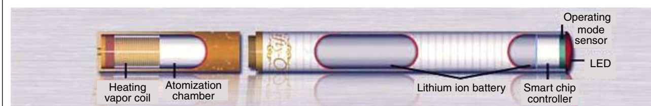
Figure 1. Basic design of an electronic cigarette.
